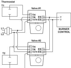
Figure-4 Typical Multiple Valve Wiring.
